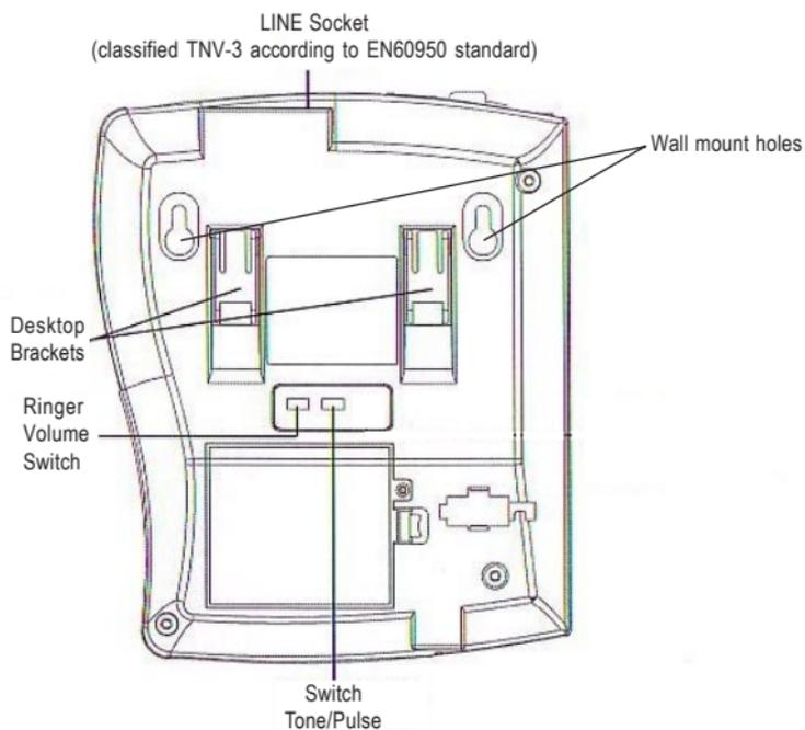
**NOTE:** Above brackets are in wall mounting state, if you wish to put your telephone on the desktop, please turn around the brackets on the desktop state as below:
